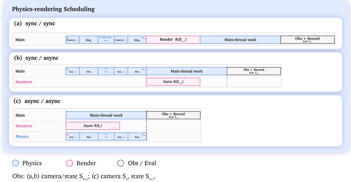
Figure 17 Physics-render scheduling in Mana. (a) sync/sync serializes physics and rendering. (b) sync/async overlaps R(S_{n+1}) with main-thread work. (c) async/async overlaps R(S_n) with physics advancing to S_{n+1} ; camera observations use S_n , while state observations and evaluation use S_{n+1} .
